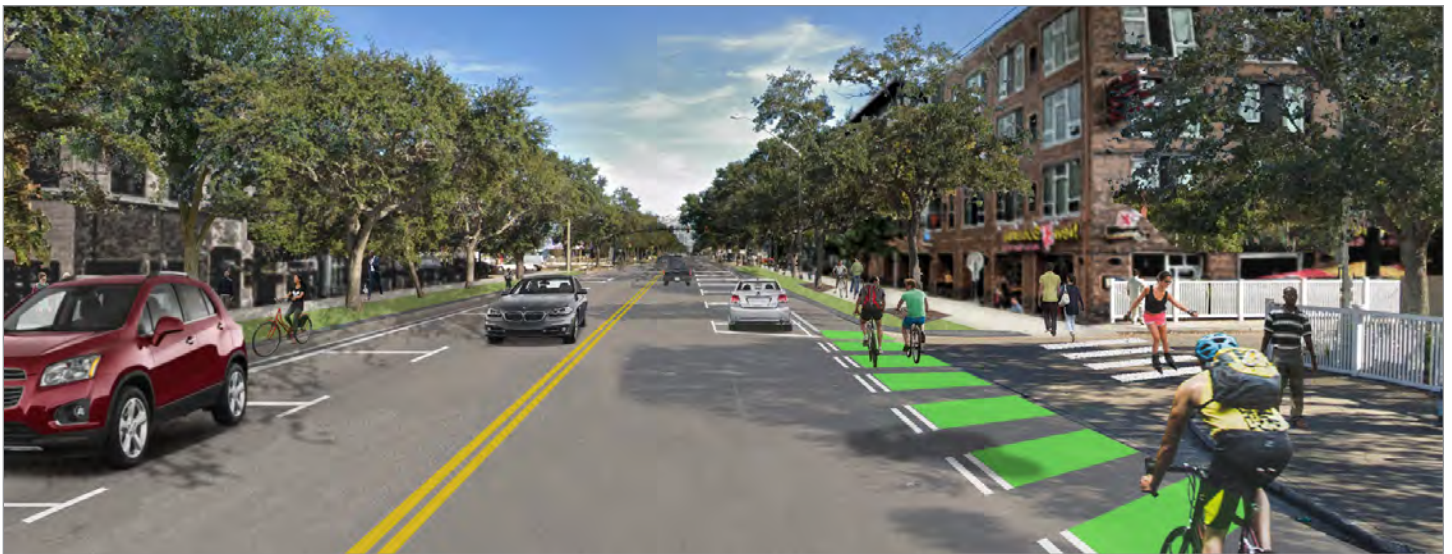
CONCEPT | Recommendations for Central Avenue looking East 31st Street: On-street Parking and Buffered Bike Lanes
